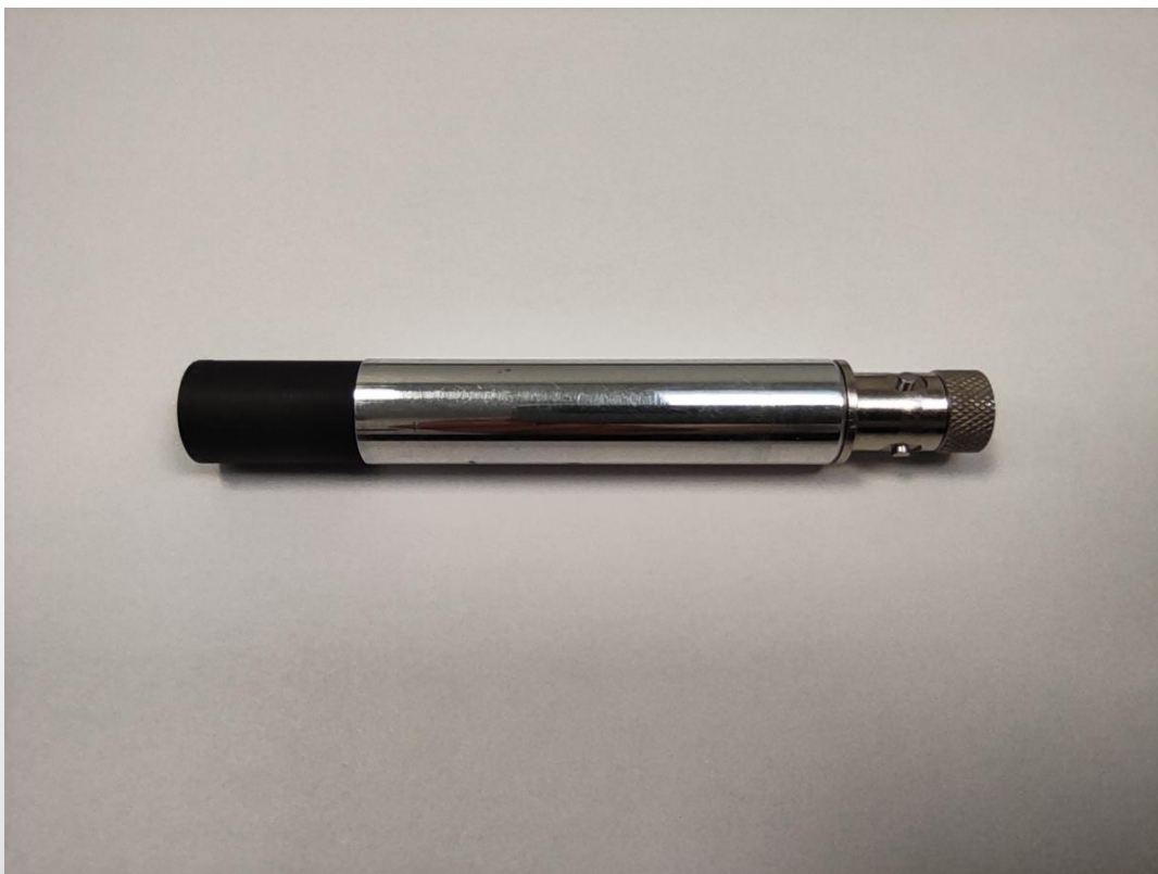
The GUM-DW3 graphite ionization chamber.
